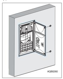
**2** - Remove the mobile part (**d**) of the power unit.
