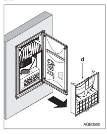
**3** - Loosen knob (e) and remove the filter cartridge to be cleaned.
