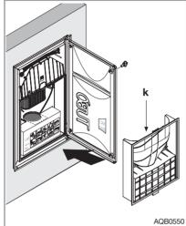
6 - Remove any dirt from the filter cartridge walls using the central vacuum system.
